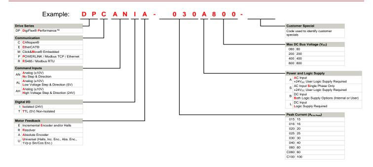
DigiFlex $\otimes$  Performance $^{\text{TM}}$  series of products are available in many configurations. Note that not all possible part number combinations are offered as standard drives. All models listed in the selection tables of the website are readily available, standard product offerings.
