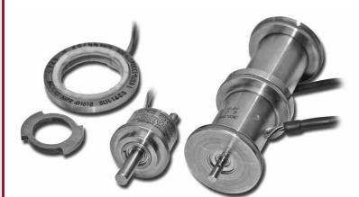
A Rotary Variable Differential Transformer (RVDT) is an electromechanical transducer that provides a variable alternating current (AC) output voltage that is linearly proportional to the angular displacement of its input shaft. When energized with a fixed AC source, the output signal is linear within a specified range over the angular displacement.
