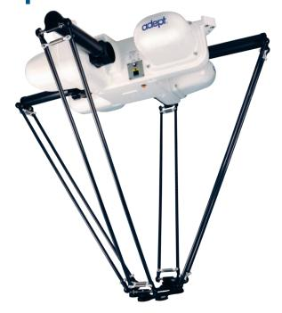
The Adept Quattro s800H is a high speed and high performance parallel robot with an extended-reach of 1.6 m, designed for high-speed applications in picking, packing, assembly, and material handling. The patented four-arm design, advanced control algorithms, and large work envelope make the Quattro s800H the ideal overhead-mount robot for smooth motion, high-throughput applications. The Quattro s800H is powered by ultra-compact controls and embedded amplifiers, minimizing the footprint.
