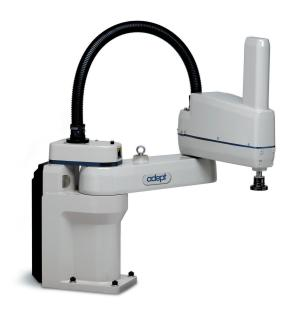
The Adept Cobra<sup>™</sup> i600 robot is an affordable, high-performance SCARA robot system for mechanical assembly, material handling, packaging, machine tending, screw driving, and many other applications that require fast and precise automation. With a built-in amplifier and motion controller, the Adept Cobra i600 delivers high footprint efficiency and is part of the industry's only line of self-contained, standalone SCARA robots.
