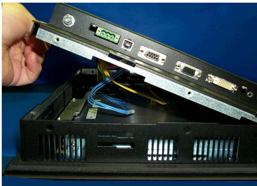
Figure 4-1: Removing the 15" Monitor Back Cover
