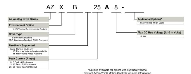
ADVANCED Motion Controls AZ series of servo drives are available in many configurations. Note that not all possible part number
