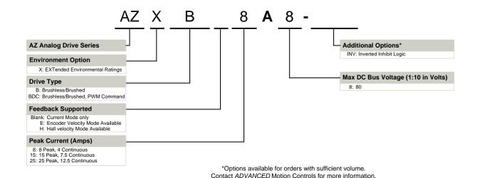
ADVANCED Motion Controls AZX series of servo drives are available in many configurations. Note that not all possible part number combinations are offered as standard drives. All models listed in the selection tables of the website are readily available, standard product offerings.
