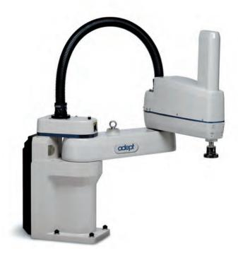
The Adept Cobra<sup>™</sup> i800 robot is an affordable, high-performance SCARA robot system for mechanical assembly, material handling, packaging, machine tending, screw driving, and many other applications that require fast and precise automation. With a built-in amplifier and motion controller, the Adept Cobra i800 delivers high footprint efficiency and is part of the industry's only line of self-contained, standalone SCARA robots.
