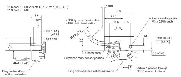
NOTE: RGH20/RESR only shown. For detailed installation drawings, refer to relevant RGH20 Installation guide or Data sheet.
