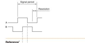
Incremental 2 channels V, and V, differential sinusoids in quadrature (90° phase shifted)
